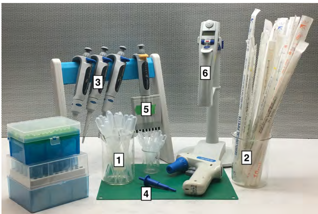
Figure 1: Common pipettes used in the lab. (1) Pasteur pipettes, (2) Graduated pipettes, (3) Adjustable Micropipettes, (4) Fixed Micropipettes, (5) Multichannel Pipette, (6) Robotic Pipette.
