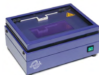
Cat. #558 Midrange UV Transilluminator 7 x 14 cm UV filter
