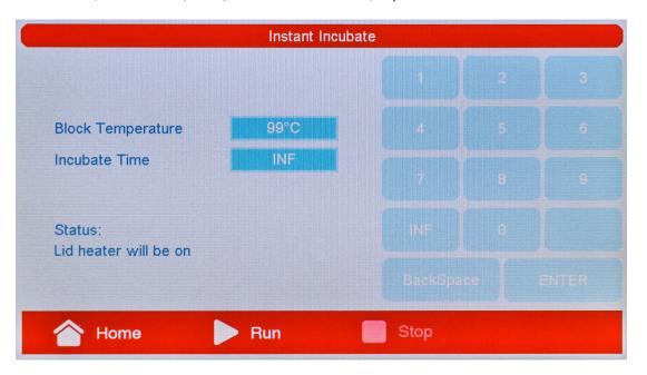
Once you have set the parameters for the hold, hit the Run button to start the incubation. After the block has reached the set temperature a timer will start to indicate the remaining time. During an incubation the options to Pause or Stop the incubation will become selectable. Tapping the Pause button will allow you to pause and then resume an incubation. The stop button will terminate an incubation.
