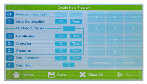
The Create New Program page allows you to edit, save, and run a new program. Note: the "Run" button will not selectable until a program has been saved.
