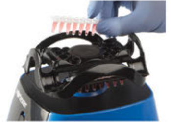
0.2 mL microfuge tubes (strip tubes) x 24 (vertically mounted)
