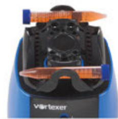
15 mL conical tubes x 2 (horizontally mounted)
