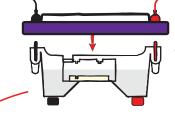
Attach safety cover & connect leads to power source to conduct electrophoresis.
