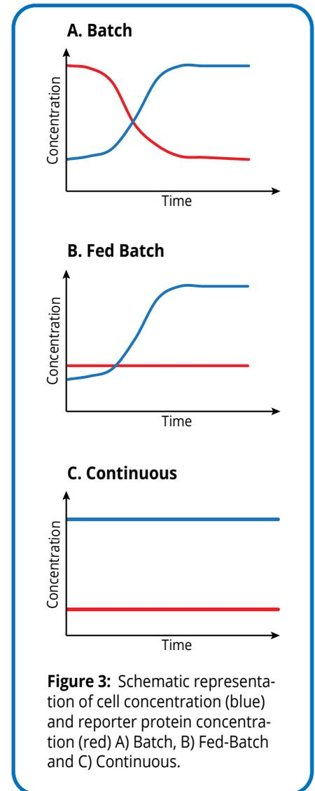
**Figure 3:** Schematic representation of cell concentration (blue) and reporter protein concentration (red) A) Batch, B) Fed-Batch and C) Continuous.
