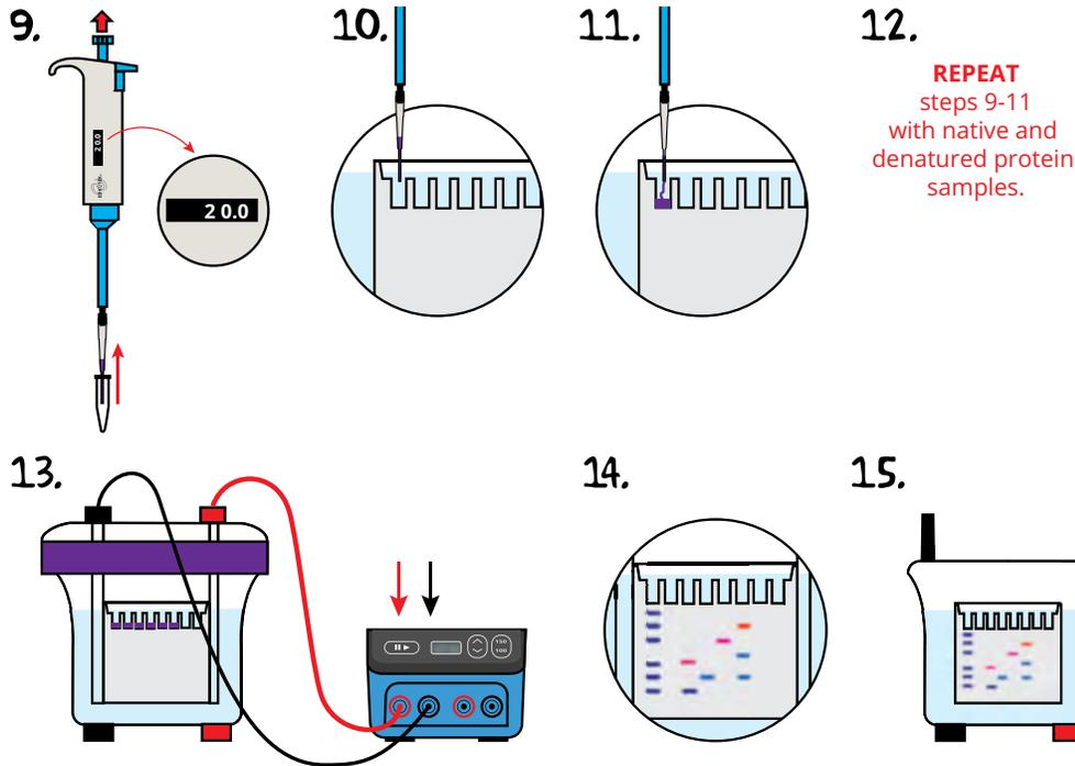
9. Using a fresh pipet tip, **MEASURE** 20 µl of the Standard Protein Marker.
