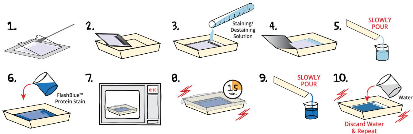
1. After electrophoresis, **LAY** the cassette down and **REMOVE** the front plate by placing a thin spatula or screwdriver at the side edge and gently lift it away from the larger back plate. In most cases, the gel will stay on the back plate. If it partially pulls away with the front plate, let it fall onto the back plate. **Handle very carefully as the thin gels are extremely fragile.**
